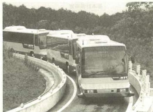
図4 IMTS (Intelligent Multimode Transit System)
